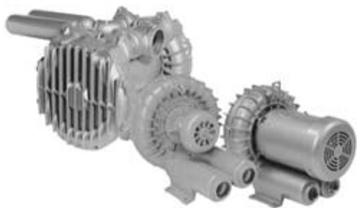
A certain amount of air slips past each impeller blade during rotation and returns to the base of a succeeding blade for reacceleration—"regenerative."
